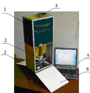
1-body, 2-actuator, 3-guide for untreated ears, 4-loading window, 5-control unit, 6-guide for cleaned ears
